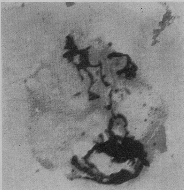
FIG. 5. Partially developed silver bromide crystal. Undeveloped portion dissolved out (Hall and Schoen).
